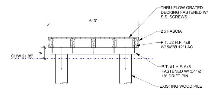
**PIER WALKWAY SECTION A** (PROPOSED) SCALE 1/2" = 1'-0"
